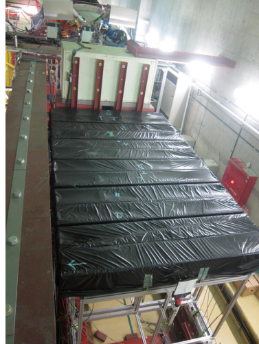
Figure 2.50: Entire view of BHPV from the downstream side. There are 16 modules implemented in the KOTO detector system at present while only 12 modules can be seen in the picture which was taken in 2013. The figure is quoted from Ref. [68].
