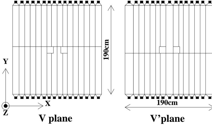
Figure 2.5: Schematic view of Trigger Hodoscopes(V, V' bank).
