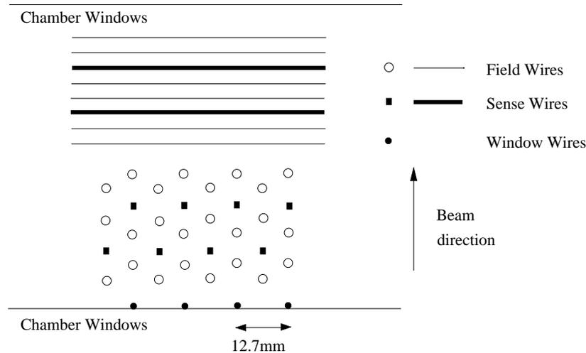
Figure 2.4: The sense and field wire geometry of the drift chamber. The field shaping wire formed a hexagonal cell with the sense wire located at the center.
