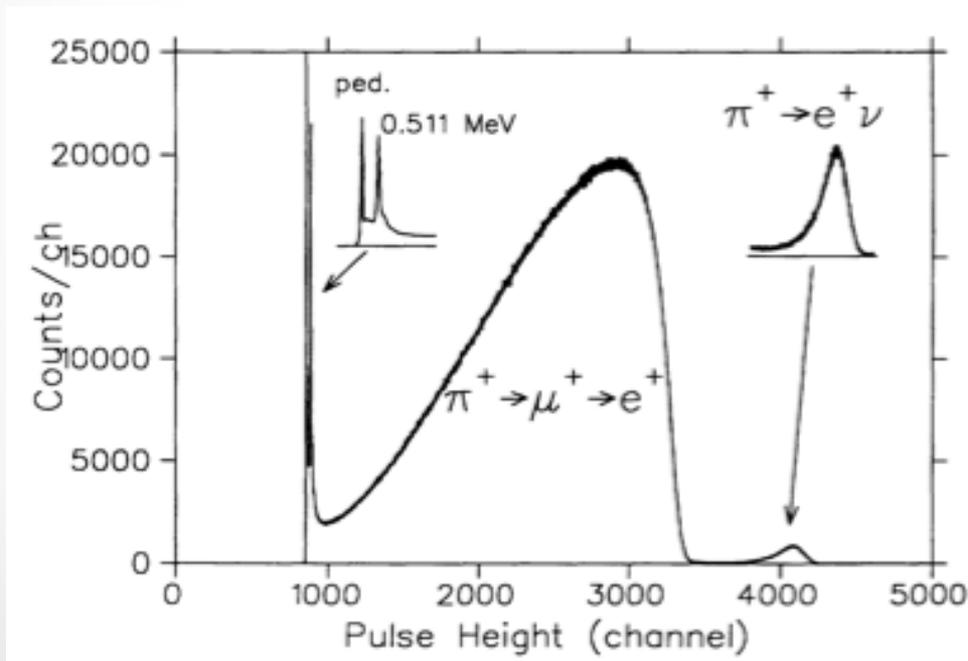
Positron's energy deposit in NaI scintillator.
