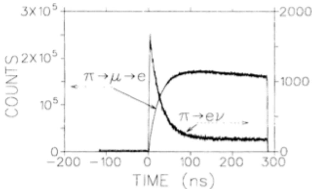
Time spectrum for upper ( $\pi \rightarrow e \nu$ ) and lower ( $\pi \rightarrow \mu \nu$ ) parts of the energy spectrum. (This figure is also previous experiment graph.)
