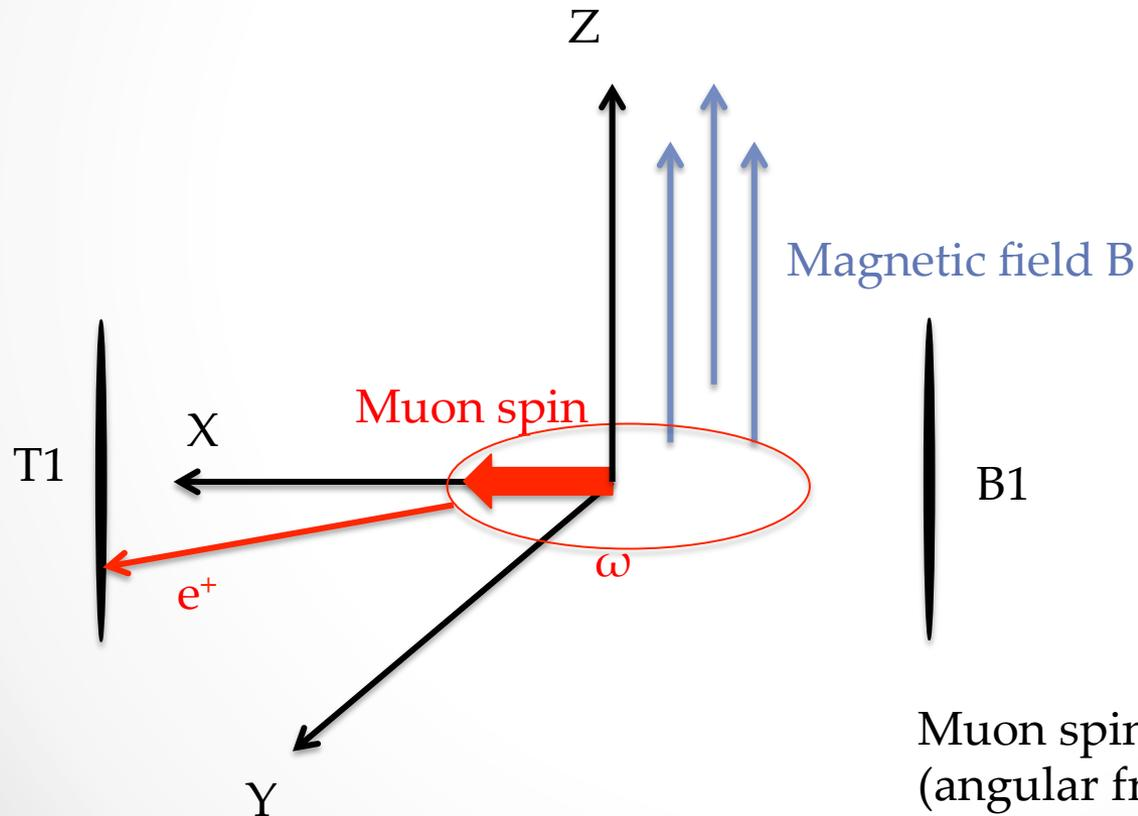
Muon spin rotates around B vertically
