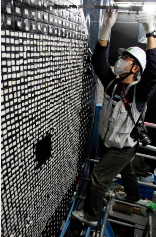
How do we prevent the crystals from flying out when the next large earthquake comes?
