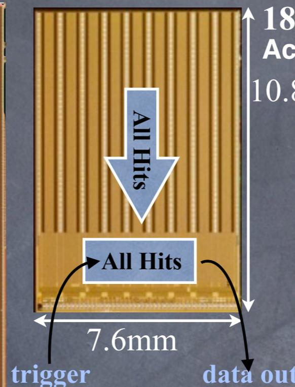
FE-I3: All hits go to periphery (column drain architecture).
