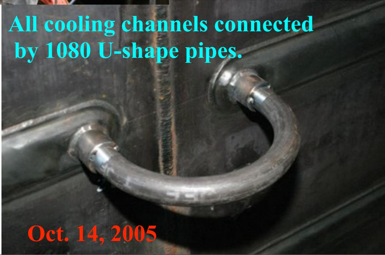
**All cooling channels connected by 1080 U-shape pipes.**
