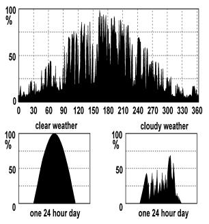
**Figure 1** Availability of Electric Power from River Hydro [STRO], Wind [WAG] and Photovoltaic [GOE] Powerplants: Restrictions and Fluctuations in Time
