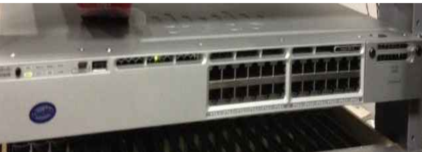
High performance network switch Cisco Catalyst WS-C3850-24T-S
