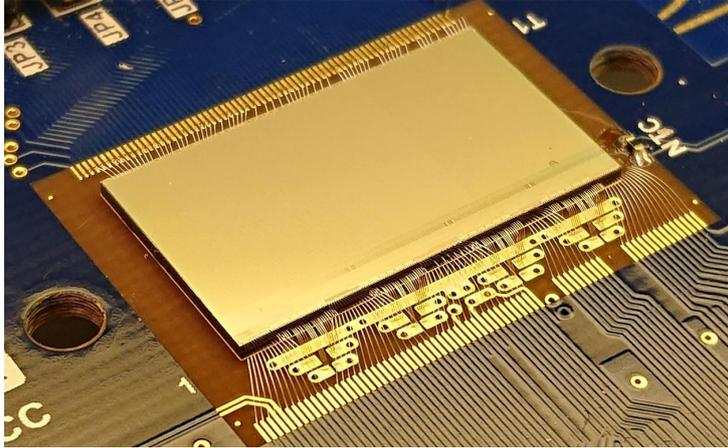
**Figure 1.8:** Picture of the RD53A ASIC, mounted on a card that permits its readout. Picture taken at the University of Bergen (Norway).
