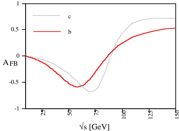
Fig.1-2 Forward-Backward Asymmetry of b/c Quark
