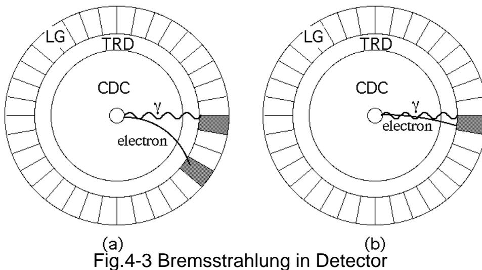
Schematic illustrations of bremsstrahlung in the detector. (a) a hard photon bremsstrahlung, (b) soft photon bremsstrahlung. In case (a), clusters of electron and photon is separated and  $E/p$  of charged track are calculated correctly as 1.0. However, in case (b), photon and charged track go into the same cluster. In this case,  $E/p$  is larger than 1.0, because the momentum of the charged particle is measured after bremsstrahlung.
