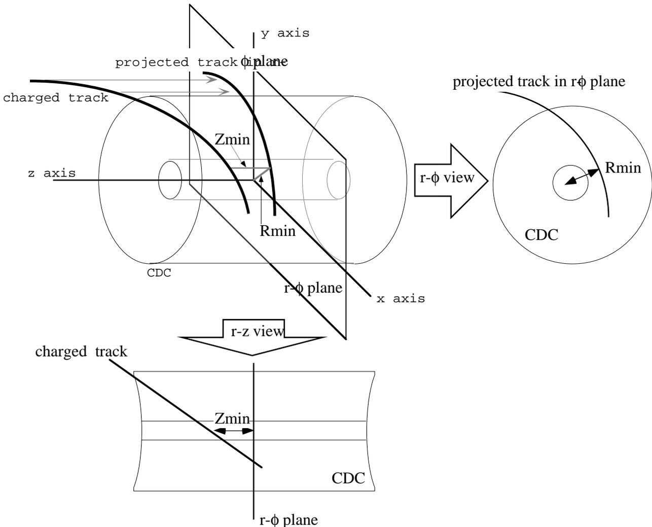
Fig.3-1 Definition of CDC Track Parameters
