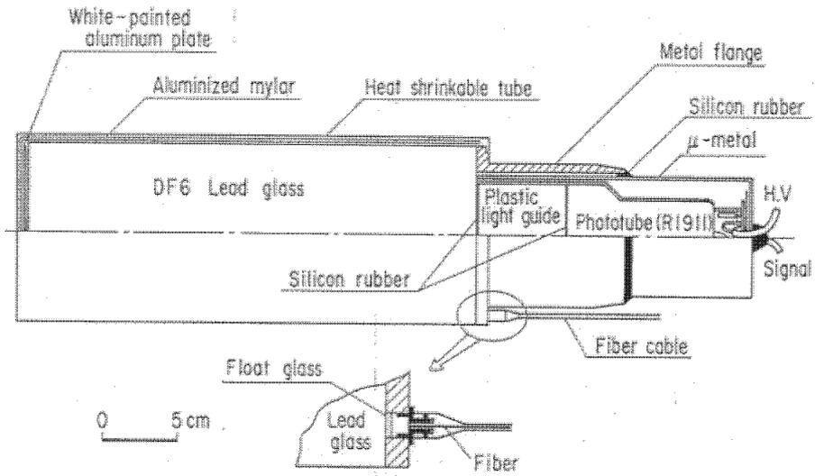
Fig.2-8b LG PMT
